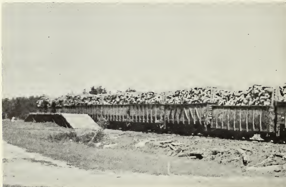
Fig. 6.--Ramps are available at many sidings to facilitate the loading of pulpwood onto rail cars. (Photo courtesy of Soo Line Railroad Co.)
